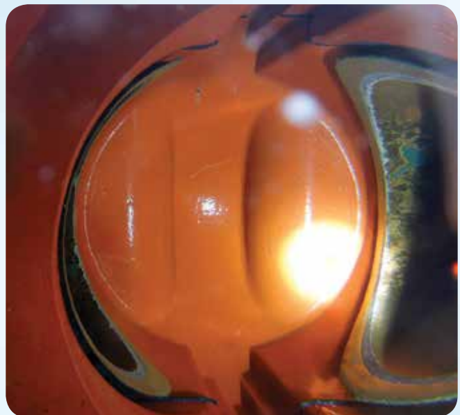
An under-pressure look of clean valve seat.
