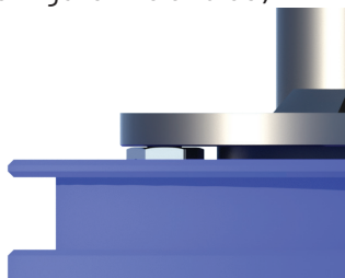
FIGURE 50 Raised Face of Insertion tool installed flush to cartridge.
