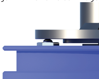
FIGURE 49 Insertion tool making contact with the auto equalization pin.
